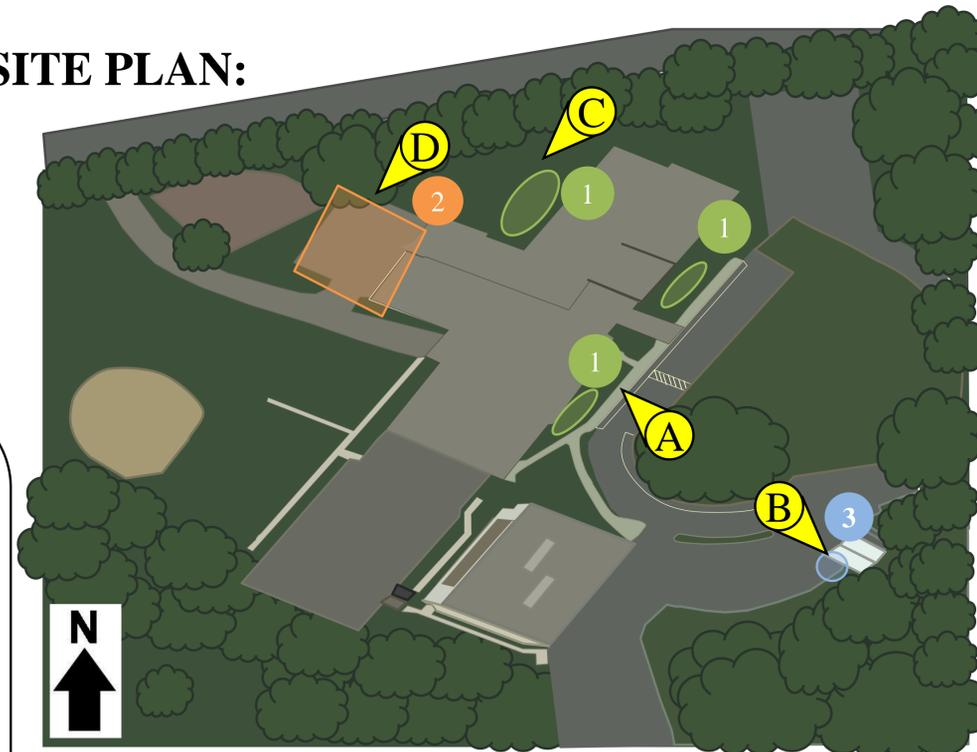
**1 BIORETENTION SYSTEM:** A rain gardens can be installed on this property to reduce sediment and nutrient loading to the local waterway and increase groundwater recharge. There are opportunities to install rain gardens in front of the school and in the rear courtyard.
